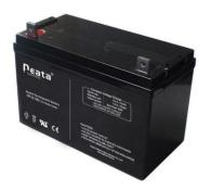
Batteries are also available in unsealed and sealed types. The unsealed types are much more common due to their lower cost. However, they do require weekly maintenance to keep their electrolyte levels above the plates inside the battery. The sealed batteries come at a premium, but do not require the maintenance, since the electrolyte is usually in a gel substance.
