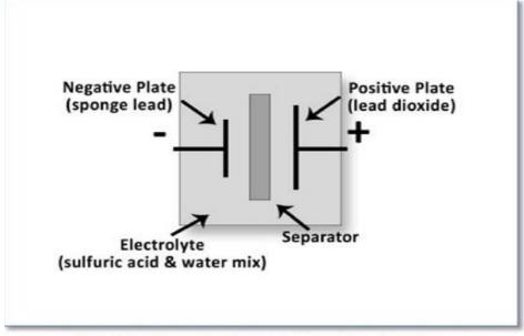
Description: Schematic diagram of a cell inside a 12v battery.
