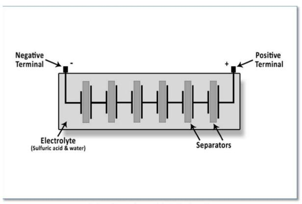
Description: Schematic diagram of the inside of a 12v battery.
