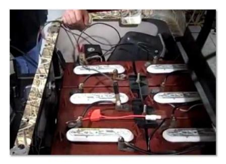
**Step 2:** Open up the battery and check if there is enough water covering all of the plates in each cell. If not, add distilled water as needed.
