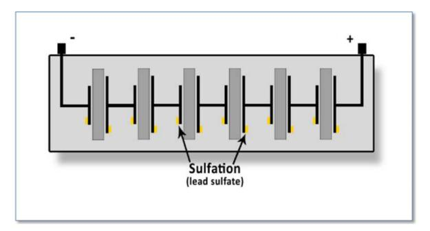
**Description**: Schematic diagram of the inside of a 12v battery that is fully charged (with minimal sulfation on the plates).
