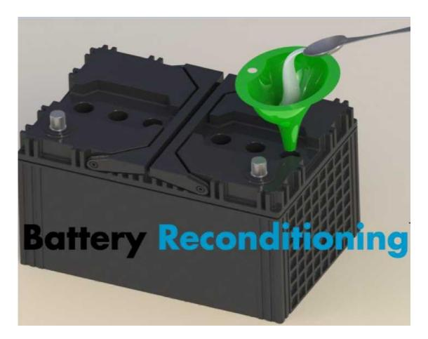
**Description:** Using a funnel and spoon to pour the right amount of Epsom Salt OR Battery Treatment Chemical into each cell.
