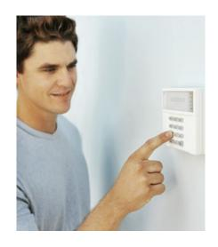
There are two overall types of monitoring: self-monitoring and professional monitoring. With self-monitoring, an alarm system with door or window sensors and possibly a motion detector is also equipped with an auto-dialer feature, and the unit is connected to a conventional landline phone line.
