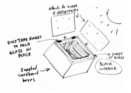
Above you have a solar oven design made with cardboard boxes, aluminum foil and a piece of window glass. Interior of the box is flat black paint.
